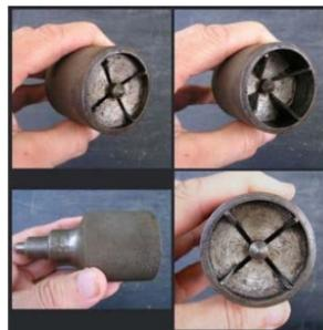
This tool, when introduced at the start of the 20<sup>th</sup> century, was a handy tool any machinist would be happy to have. It is a center punch with a retractable tapered center punch. It was specifically made to quickly find and mark the center of any diameter rod stock that fits within its punch diameter.
