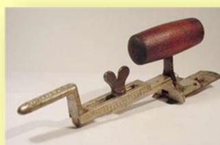
This is an old Stanley clamp gauge made of cast metal and steel with an attractive walnut handle and a nice cast iron wing nut. It is adjustable from 2 3/4 inches to 4 1/2 inches in order to guide a housewright or carpenter in placing clapboards at the right heights in relation to one another for the best protection and appearance of the siding.
