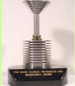
This is a 1940's 1 to 8 ounce postal weight scale made by Thompson Tool and Manufacturing Co. of Franklin Park, IL. It was fabricated from solid turned aluminum with a Bakelite base. It was usually imprinted and given as advertising gifts. No doubt the forerunner of today's imprinted pens, coffee cups and tee shirts.
